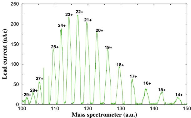
Figure 1: CSD for lead in MINIMAFIOS. Injected beam : 220 nA of  $Pb^{1+}$ .
