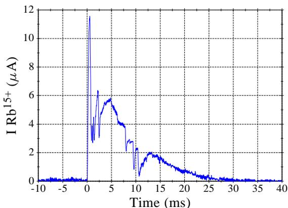
Figure 4: An  $Rb^{15+}$  peak current of  $11.5 \mu A$  is extracted for 400 nA of  $Rb^{1+}$  injected.
