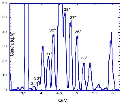
Fig. 3 – Charge state distribution for Xe, optimized for  $30^+$ .
