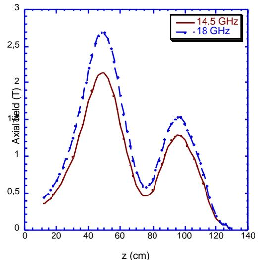
Fig. 2 – Axial magnetic field of SERSE.
