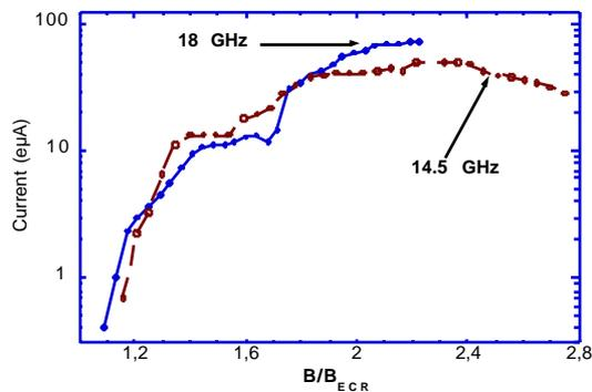
Fig. 6 –  $\text{Xe}^{27+}$  currents vs.  $B_{\text{radial}}/B_{\text{ECR}}$ .
