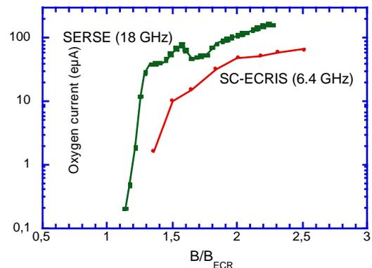
Fig. 8 –  $\text{O}^{7+}$  current vs.  $B_{\text{radial}}/B_{\text{ECR}}$ .
