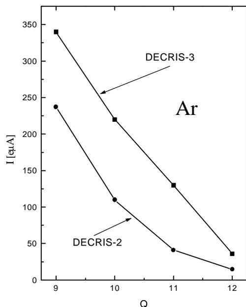
Fig. 3. Comparison of the typical ion currents from the DECRIS-3 ion source and its predecessor.
