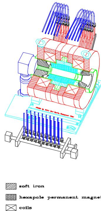
Fig. 1. Schematic overview of the DECRIS-3 ion source.
