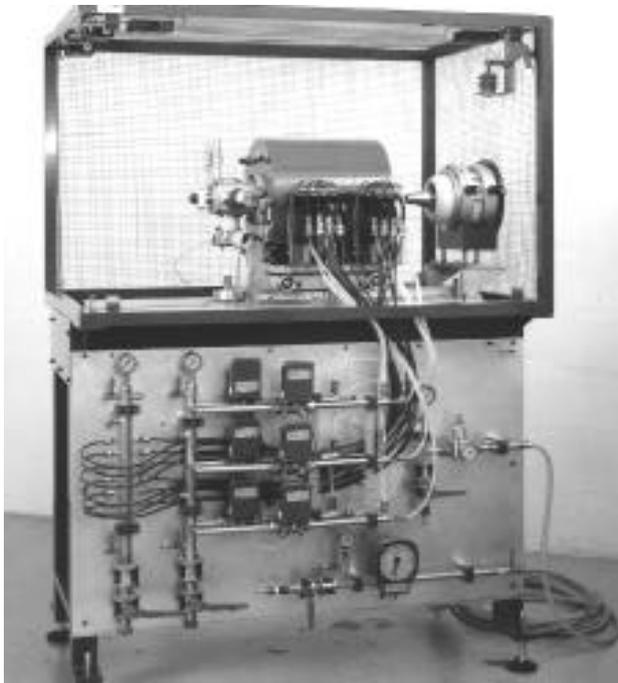
Fig. 2 – The ECR2 source on its support stand.
