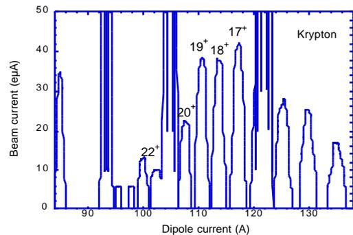
Fig. 3 – A charge state distribution, optimized for  $\text{Kr}^{22+}$ .
