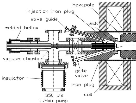
**Fig. 4:** Sketch of the modified injection side of the source.
