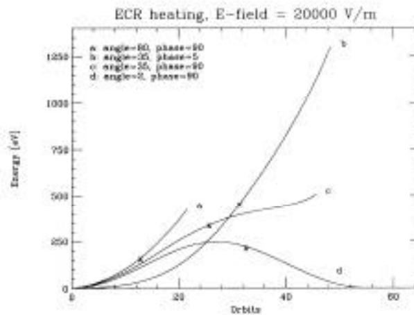
Figure 2: The energy of the electron as a function of the number of the orbits. The turning point of the electron is denoted by  $x$ . Four different angles and phases of the electron were used.
