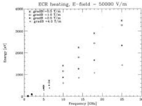
Figure 6: The energy of the electron as a function of the microwave energy when different gradients of the magnetic field were used. An initial electron energy of 1eV was used. Points correspond to the maximum energy obtained during one heating period with optimum angle and phase of the electron. The amplitude of the electric field decreases as a function of the permittivity according to equation (2).
