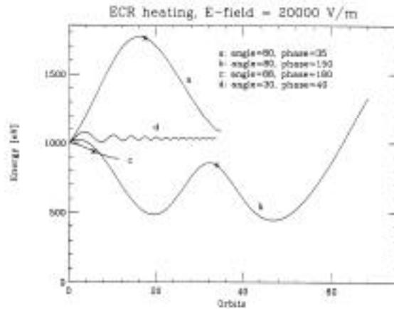
Figure 3: The energy of the electron as a function of the heating orbit numbers. The initial energy of 1 keV was used. The reflection point is denoted by x.
