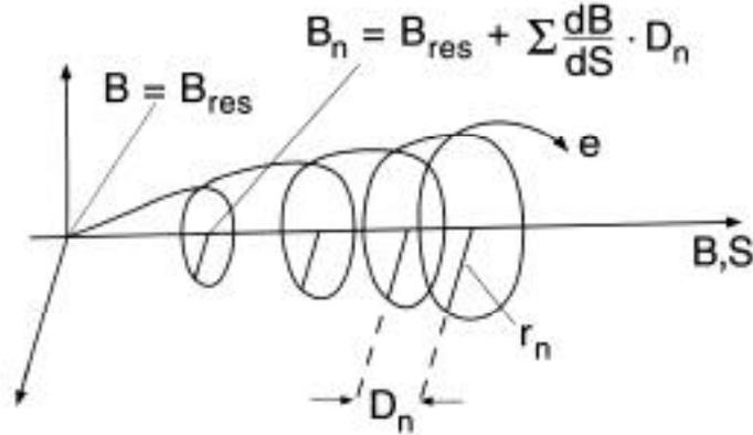
Figure 1: The trajectory of the electron that enters the resonance region from the core of the plasma. The heating of the electron starts at the point where  $B=B_{res}$ .
