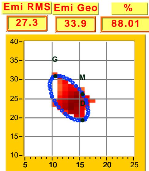
Figure 8: Emittance figure of  $Ar^+$  beam. Extraction voltage=14 kV, Einzel voltage=7kV, plasma electrode hole diameter=9 mm.
