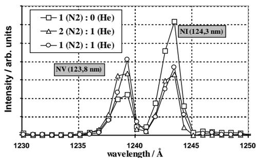
Fig. 6: Improvement of the charge state distribution with higher helium admixtures in ECRIS II
