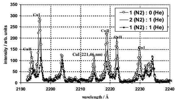
Fig. 3: VUV spectra at different gas mixture ratios
