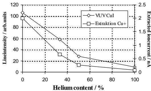
Fig. 4: Comparison of CuI (221,5 nm) emission line and extracted Cu<sup>+</sup> ion current
