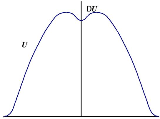
Figure 1. Plasma potential  $U$  with potential dip  $DU$
