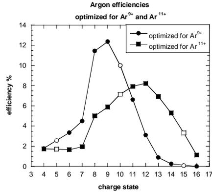
Fig.1 Ionization efficiency distribution for argon spectra optimized on Ar<sup>9+</sup> and Ar<sup>11+</sup> with oxygen as support gas. The open symbols indicate the mixed ion species.
