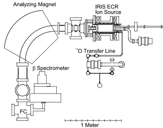
Fig. 6 Schematic of the new exotic ion beam test stand and the  $^{14}\text{O}$  experiment.
