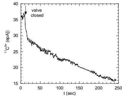
Fig.5 Current decay for a  $^{11}C^{6+}$  ion beam after extraction from the cyclotron after 12 minutes of continuous release from the cryogenic trap
