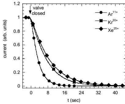
Fig.2 Normalized beam current decay for selected charge states for a few noble gases with the LBNL AECR-U ion source.
