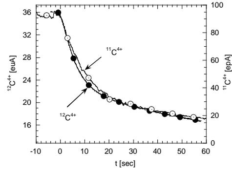
Fig.4 Current decay for a  $^{11}C^{4+}$  ion beam after extraction from the cyclotron during the first minute of activity release from the cryogenic trap in comparison with the stable  $^{12}C^{4+}$  ion beam decay.
