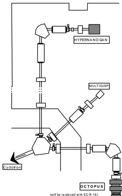
Fig. 1 Schematic layout of ECR ion sources for the cyclotron.
